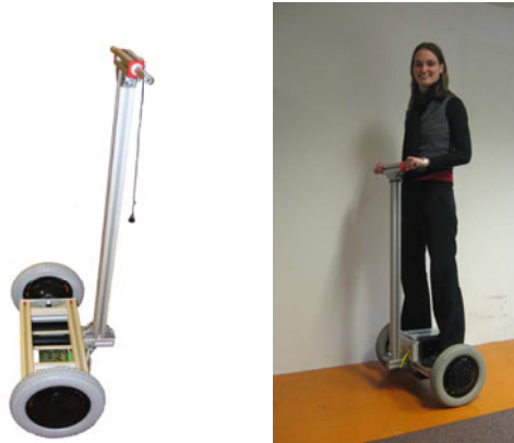
Fig. 6. The ChessWay personal transporter
